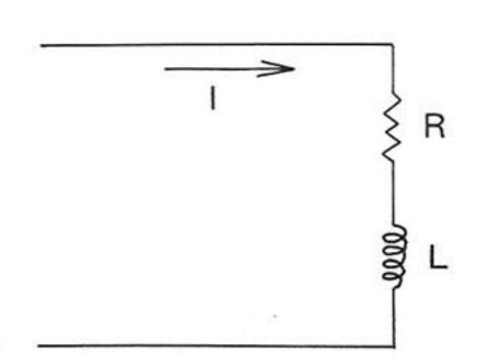
Determine the ratio of electric current (i) in the RL circuit (R =  $20\Omega$ , L = 3H) shown left 0.2 second after the switch is closed.
